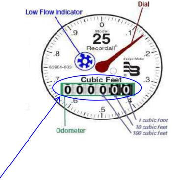
This is your meter reading. Please write down the six (6) numbers as you see them, from left to right. Water meters are typically located in basements, under kitchen sinks, or in laundry rooms near hot water tanks.
