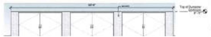
10 DUMPSTER ELEVATION (TYP.) 3/8" = 1'-0"
