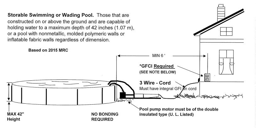
**STORABLE POOLS ONLY.** The type of pump suitable for use with storable pools has a 25' flexible cord and attachment plug. It is marked:
